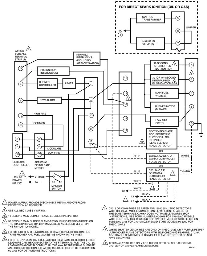
Fig. 15. Sample block diagram of field wiring for R4140G1007, R4140G1015 and R4140G1006 Programmers.
